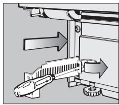
■ To adjust the depth (recess) of the toekick, release the tension on the spring clips as shown, and push the mounting brackets in as far as possible.
